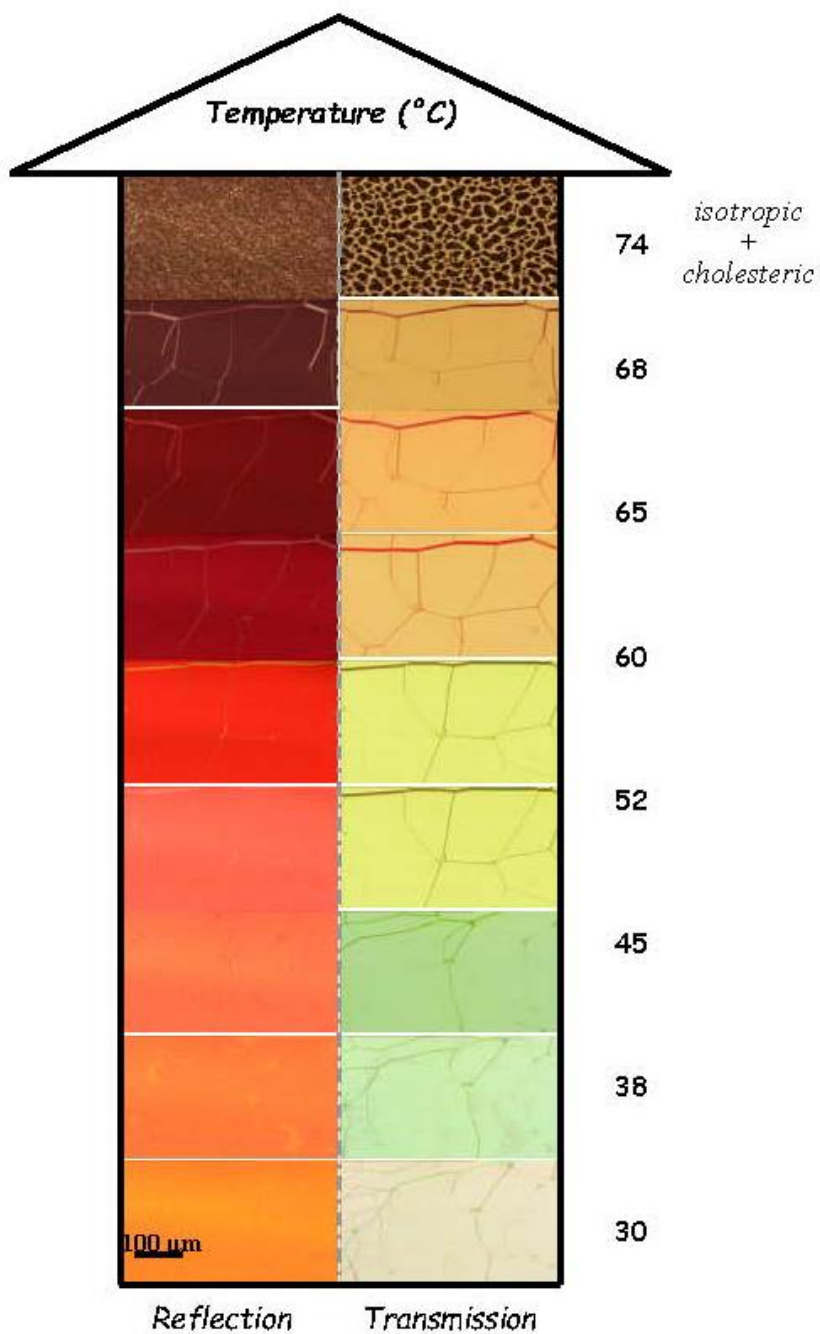
FIGURE 1.- Polymorphism of the CLC blend before curing: optical textures at different temperatures (crossed polarizers).
