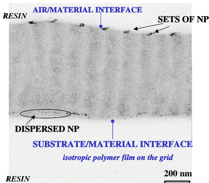
**Fig. 2.** TEM micrograph of a cross-section of cholesteric LC SR doped with np.
