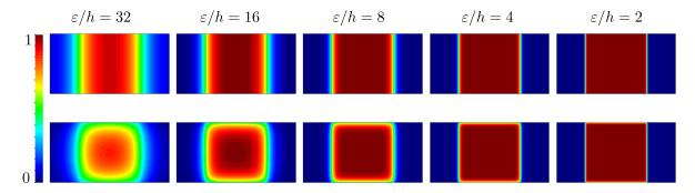
FIGURE 5. (Upper row) values of the regularized characteristic function  $v_{\varepsilon}^{\text{Neu}}$ ; (lower row) values of the regularized characteristic function  $v_{\varepsilon}^{\text{Rob}}$  in the validation example of Section 6.1.
