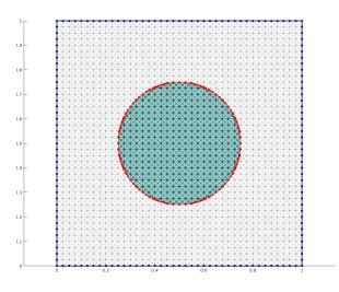
FIGURE 7. Setting of the numerical experiment conducted in Section 6.2. The shape  $\Omega$  (in blue) is not explicitly discretized in the mesh of D, but it is represented as the negative subdomain of a "level set function".
