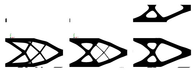
FIGURE 13. Several iterations of the minimization of a weighted sum of the compliance and the perimeter of a 2d cantilever under a volume constraint in Section 6.4.2. (Upper row) the relative perimeter functional is used; (lower row) the total perimeter functional is used.
