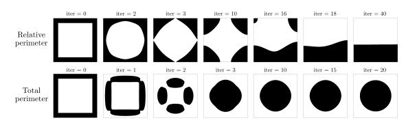
FIGURE 11. Several snapshots of the evolution of the design in the perimeter minimization example under volume constraint considered in Section 6.3; (upper row) the relative perimeter functional  $P_{\varepsilon}^{\text{Neu}}$  is used; (lower row) the total perimeter functional  $P_{\varepsilon}^{\text{Rob}}$  is used.
