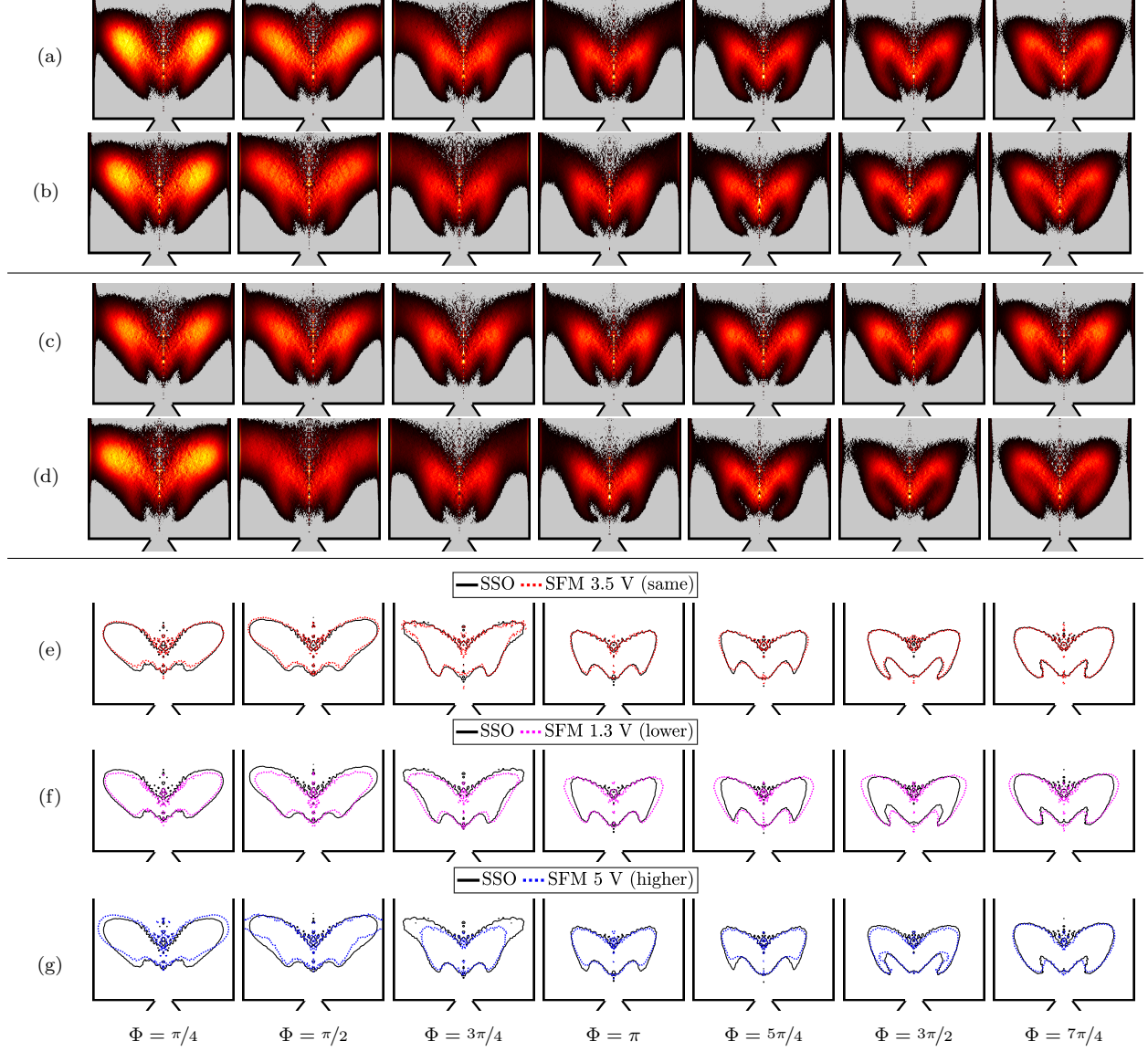
Figure 2: (a-d) Phase-averaged, Abel-transformed flame images shown in false colors. Light intensity of OH* chemiluminescence is obtained at different phase instants of the acoustic cycle using an intensified camera. (a) Images obtained under SSO at a frequency f_0 = 533 Hz. I'_{\text{OH}^*}/\overline{I_{\text{OH}^*}} = 28.9\% . (b-d) Images corresponding to SFM at the frequency of SSO. (b) The forcing amplitude matches that observed during SSO ( I'_{\text{OH}^*}/\overline{I_{\text{OH}^*}} = 30.4\% ). (c) The forcing amplitude is lower than that observed during SSO ( I'_{\text{OH}^*}/\overline{I_{\text{OH}^*}} = 14.2\% ). (d) The forcing amplitude exceeds that observed during SSO ( I'_{\text{OH}^*}/\overline{I_{\text{OH}^*}} = 37.8\% ). (e-g) Flame isocontours determined by Otsu thresholding method for SSO (solid line in (e-g)) and three levels of SFM (same—dotted line in (e), lower—dotted line in (f), and higher—dotted line in (g) fluctuation level compared to SSO).
