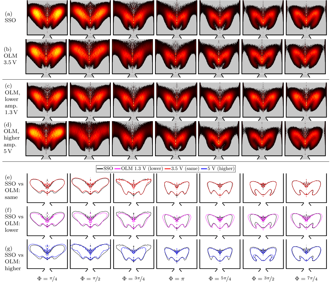
Figure 2: Phase-averaged, Abel-transformed flame images shown in false colors. Light intensity of \text{OH}^* chemiluminescence is obtained at different phase instants of the acoustic cycle using an intensified camera. (a) Images obtained under self-sustained oscillations (SSO) at a frequency f_0 = 533 Hz. I'_{\text{OH}^*}/\bar{I}_{\text{OH}^*} = 28.9\% . (b-d) Images corresponding to open-loop modulation (OLM) at the frequency determined under SSO. (b) The forcing amplitude matches that observed during SSO ( I'_{\text{OH}^*}/\bar{I}_{\text{OH}^*} = 30.4\% ). (c) The forcing amplitude is lower than that observed during SSO ( I'_{\text{OH}^*}/\bar{I}_{\text{OH}^*} = 14.2\% ). (d) The forcing amplitude exceeds that observed during SSO ( I'_{\text{OH}^*}/\bar{I}_{\text{OH}^*} = 37.8\% ). (e-g) Flame isocontours determined by Otsu thresholding method for SSO and three levels of OLM (same, lower, and higher fluctuation level compared to SSO).
