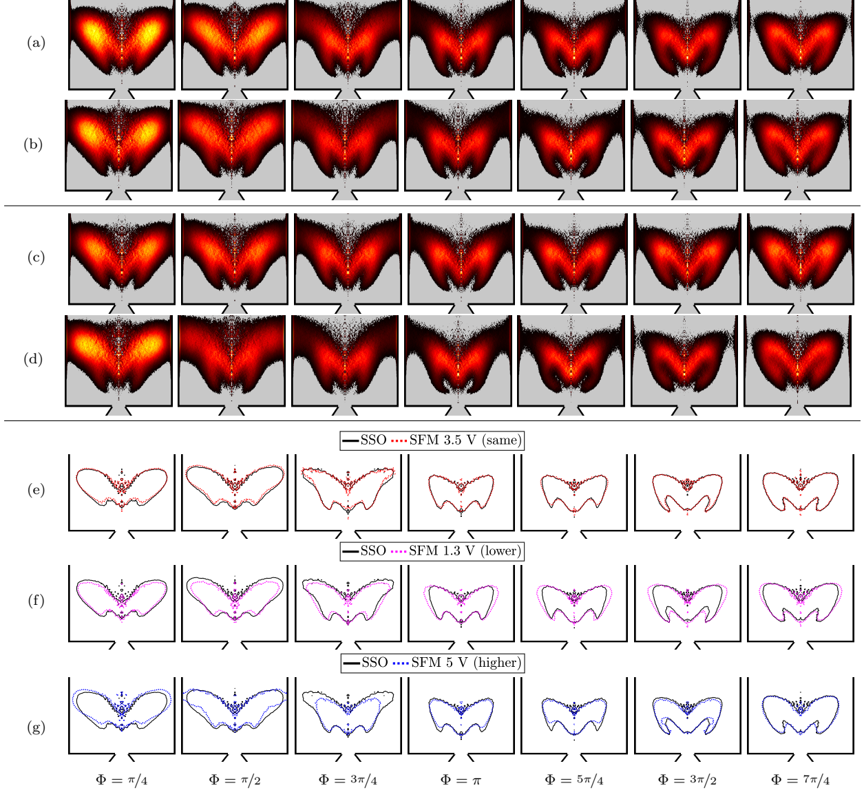
Figure 2: (a-d) Phase-averaged, Abel-transformed flame images shown in false colors. Light intensity of \text{OH}^* chemiluminescence is obtained at different phase instants of the acoustic cycle using an intensified camera. (a) Images obtained under SSO at a frequency f_0 = 533 Hz. I'_{\text{OH}^*}/I_{\text{OH}^*} = 28.9\% . (b-d) Images corresponding to SFM at the frequency of SSO. (b) The forcing amplitude matches that observed during SSO ( I'_{\text{OH}^*}/I_{\text{OH}^*} = 30.4\% ). (c) The forcing amplitude is lower than that observed during SSO ( I'_{\text{OH}^*}/I_{\text{OH}^*} = 14.2\% ). (d) The forcing amplitude exceeds that observed during SSO ( I'_{\text{OH}^*}/I_{\text{OH}^*} = 37.8\% ). (e-g) Flame isocontours determined by Otsu thresholding method for SSO (solid line in (e-g)) and three levels of SFM (same—dotted line in (e), lower—dotted line in (f), and higher—dotted line in (g) fluctuation level compared to SSO).
