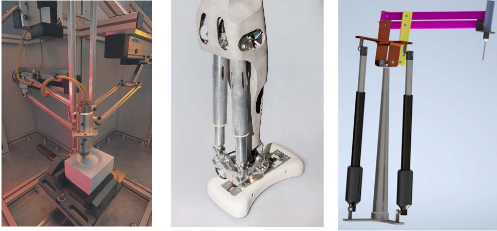
Figure 1: The parallel mechanisms used in different applications. From left: Orthoglide used in milling operations [19], active ankle used in humanoids [24], RCM mechanism used in surgery [12]
