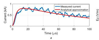
**Fig. 7** *Current and electric field waveforms at 15 km for MM2* (a) Current, (b) Electric field
