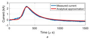
Fig. 13 Current and electric field waveforms at 15 km for MICC2 (a) Current, (b) Electric field
