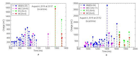
**Fig. 4** Transferred charge associated with each pulse as a function of the time of occurrence in the flashes that occurred on 4 August 2016 at (a) 23:57, (b) on 23:52
