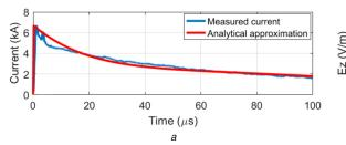
**Fig. 8** *Current and electric field waveforms at 15 km for RS1* (a) Current, (b) Electric field
