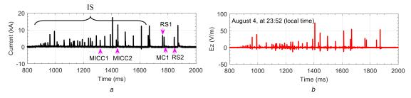
Fig. 1 Overall current and electric field waveforms measured at 15 km (a) Current, (b) Electric field. The waveforms are associated with an upward negative flash initiated from the Säntis Tower on 4 August, at 23:52. The pink arrows in the left panel show five of the eight pulses used in Section 4
