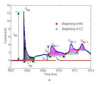
the time integral of the MC pulse above the  $I_{CC}$  during  $T_{M}$  (the pink-shaded area in Fig. 14*b*). The evaluation of the charge in two additional MC pulses is also illustrated in Fig. 14*b*.
