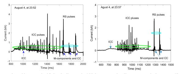
**Fig. 3** *Current waveforms of the two considered flashes after filtering with a 1-kHz low-pass, zero-phase filter to accentuate the slower varying ICC and the CC. The green coloured ellipse groups the ICC pulses and the cyan blue coloured ellipse groups the RSs and MCs pulses*
