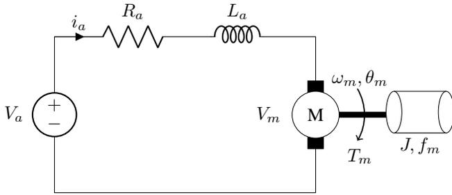
Fig. 1. Electrical equivalent circuit of PMDC motor.
