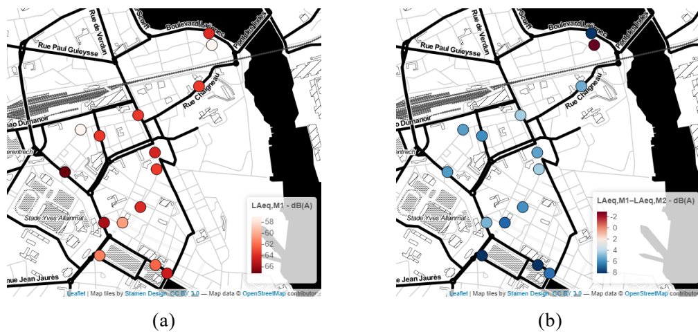
403 Figure 5 - For the 15 stations, (a) the pre-lockdown L_{Aeq,M1} and (b) its difference with the period 404 during the lockdown L_{Aeq,M1} - L_{Aeq,M2} .
