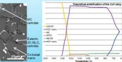
1050 Micrograph (Scanning Electron Microscope in Back Scattered Electrons mode) of the as-cast microstructure of the CoY alloy (left side) and theoretic solidification sequences plotted from Thermo-Calc calculations' results (on the right)
