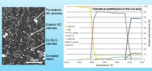
Micrograph (Scanning Electron Microscope in Back Scattered Electrons mode) of the as-cast microstructure of the CoX alloy (left side) and theoretic solidification sequences plotted from Thermo-Calc calculations' results (on the right)
