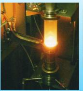
The second alloy ("CoY") elaborated in laboratory by targeting the chemical composition of a second commercial alloy; obtained comp.\*: Co(bal.)-24.1Cr-10.3Ni-0.6\*\*C-4.0Ta-0.05Ti-7.4W-0.3Zr
