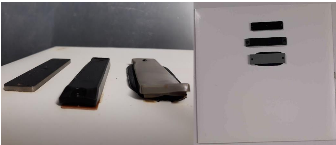
Fig. 4. RFID UHF tags after 200 hours of thermal cycling (right) and after 4000 hours of damp heat testing (left)
