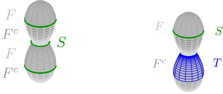
Figure 2: Expected minimizers of  $\mathcal{E}_0$  for  $\beta \ll 1$  (left) and intermediate  $\beta$  (right). For small  $\beta$  the line  $S$  has the tendency to stick to  $\mathcal{M}$  and optimize  $F$ , thus no  $T$  appears. For larger  $\beta$  one may find a configuration as depicted on the right, i.e. the energy is decreased by joining two parts of  $S$  by a surface  $T$  glued to  $\mathcal{M}$ .
