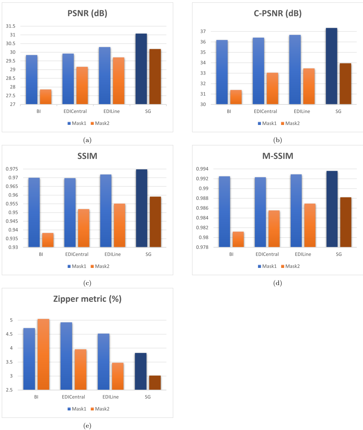
Fig. 20: Averaged performances of reconstruction methods in terms of (a) PSNR applied on the CFA image and (b) C-PSNR, (c) SSIM, (d) M-SSIM, and (e) Zipper Metric applied on the color image. Results are computed on the Kodak database [1], the McMaster database [33] and the HDR+ burst [25] for the Mask1 and the Mask2. For each mask, the best solution is highlighted in dark.
