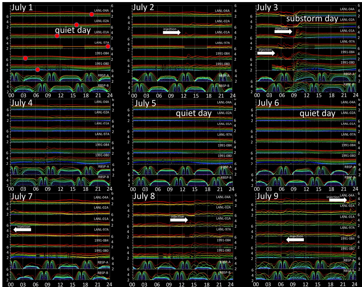
882 Figure 2: LANL-GEO (from top to bottom: LANL-04A, LANL-02A, LANL-01A, LANL-97A, 883 1994-084, 1991-080) and Van Allen Probes (RBSP B and RBSP A) survey electron flux 884 from 1 to 10 July 2014 with one panel per day. This figure shows rather quiet days (on 885 July 1, 5, 6) and mild (on July 2, 4, 7) to moderate (on July 3, 8, 9) perturbations from 886 substorm activity. White arrows point to some of the main injections. (red circle) Local 887 MLT midnight for each LANL-GEO satellite changes by less than five minutes during the 888 10-day period (1991-080: 6.33, 1991-084: 3.33, LANL-97A: 23.38, LANL-01A: 11.29, 889 LANL-02A: 15.43, LANL-04A: 19.53).
