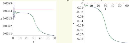
The flatness planned curve is in red, the integration with feed-back in darkblue and the generalized flatness curve in green.
