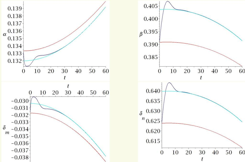
The flatness planned curve is in red, the integration with feed-back in dark blue and the generalized flatness curves in green.
