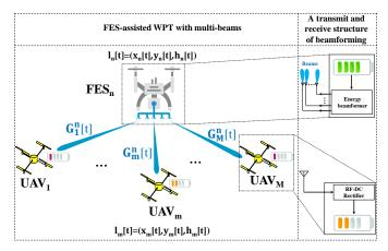
Fig. 4: Channel modeling of FES-enabled charging process.
