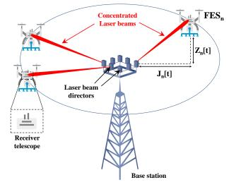
Fig. 3: Channel modeling of BS-enabled loading process.
