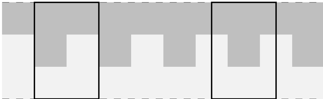
Figure 10: Periodic microstructure: choice of non-symmetric RVE vs. symmetric RVE.
