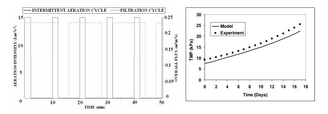
Fig. 6- Experiment C (superscript 0 expresses in influent): qa= 15 L/(m<sup>2</sup>s), tf= 12 min, tid= 4 min, Int<sub>CB</sub>= 8 min, t<sub>CB</sub>= 2min,  $X_{SST}^{0}$ = 62 mg/L,  $X_{SST}$ = 6500-9300 mg/L,  $S_{S}^{0}$ = 130 mgCOD/L,  $S_{SMP}^{0}$ = 40 mgCOD/L,  $X_{S}^{0}$ = 80 mgCOD/L,  $X_{I}^{0}$ = 24 mgCOD/L,  $S_{I}^{0}$ = 22 mgCOD/L, SRT= 50 days.
