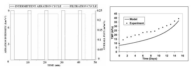
Fig. 4- Experiment A (superscript 0 expresses in influent): qa= 9 L/(m<sup>2</sup>s), tf= 12 min, tid= 4 min, Int<sub>CB</sub>= 8 min, t<sub>CB</sub>= 2min,  $X_{SST}^{0}$ = 65 mg/L,  $X_{SST}$ = 6500-9500 mg/L,  $S_S^{0}$ = 230 mgCOD/L,  $X_S^{0}$ = 100 mgCOD/L,  $X_I^{0}$ = 28 mgCOD/L,  $S_I^{0}$ = 38 mgCOD/L,  $S_{SMP}^{0}$ = 50 mgCOD/L, SRT= 50 days.
