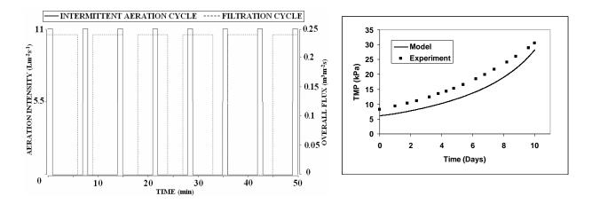
Fig. 5- Experiment B (superscript 0 expresses in influent): qa= 11 L/(m<sup>2</sup>s), tf= 6 min, tid= 3 min, Int<sub>CB</sub>= 6 min, t<sub>CB</sub>= 1min,  $X_{SST}^{0}$ = 40 mg/L,  $X_{SST}$ = 4000-4600 mg/L,  $S_S^{0}$ = 110 mgCOD/L,  $X_S^{0}$ = 90 mgCOD/L,  $X_I^{0}$ = 28 mgCOD/L,  $S_I^{0}$ = 25 mgCOD/L,  $S_{SMP}^{0}$ = 23 mgCOD/L, SRT= 40 days.
