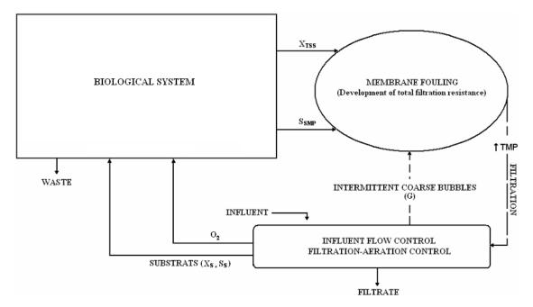
Fig.1- Conceptual schematic of developed model for SMBR
