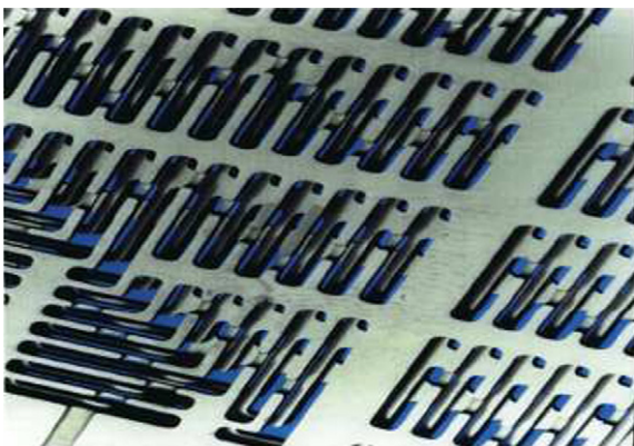
Fig. 17. Layers of slotted plates forming flow paths [51].
