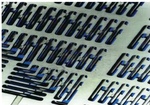
Fig. 17. Layers of slotted plates forming flow paths [51].
