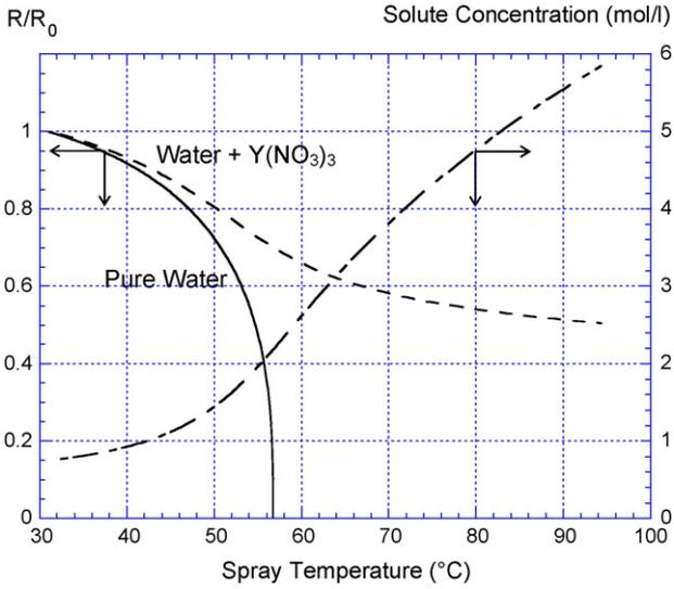
Fig. 5. Variation of the dimensionless droplet radius for pure water and water +  $Y(\text{NO}_3)_3$  and of the solute concentration vs. spray temperature.
