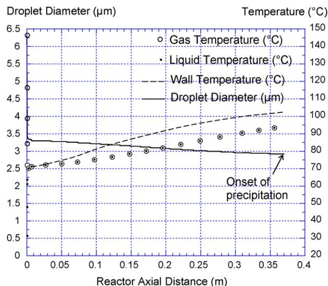
Fig. 9. Variation of the droplet radius, gas and liquid temperatures along the reactor axis for water +  $\text{Y}(\text{NO}_3)_3$ — $Fv_a = 5 \text{ m}^3 \text{ h}^{-1}$  STP,  $Fv_w = 0.581 \text{ h}^{-1}$  STP,  $d_0 = 5.2 \text{ }\mu\text{m}$ .
