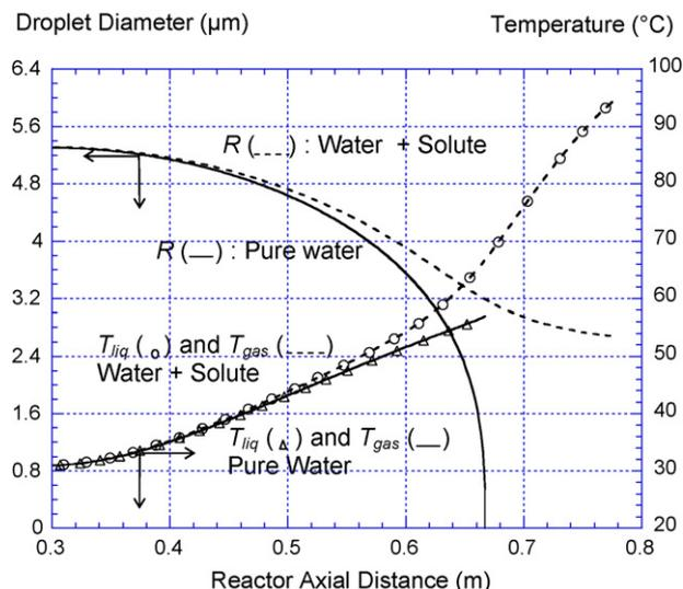
Fig. 3. Variation of the droplet diameter, gas and liquid temperatures along the reactor axis for pure water and water +  $\text{Y}(\text{NO}_3)_3$ — $F_{v_a} = 3.5 \text{ m}^3 \text{ h}^{-1}$  STP,  $F_{v_w} = 0.41 \text{ h}^{-1}$  STP,  $d_0 = 5.3 \text{ }\mu\text{m}$ .
