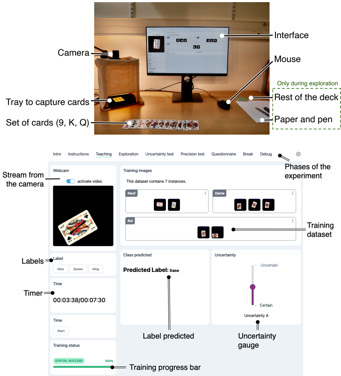
Fig. 5. Top: The setup includes a screen, mouse, and camera stand for recording individual cards. Participants have access to the 12 training cards, the rest of the deck, paper and pens. Bottom: The application displays the live webcam feed, training set, prediction, uncertainty estimation and a series of tabs associated with each step of the experiment. The above interface is not shown in full screen for legibility. During the experiment, the different components are arranged in the same way but in full screen format.
