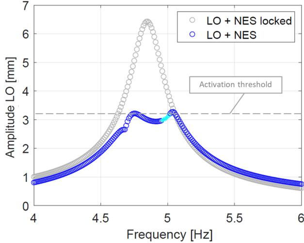
Figure 15: Evolution of the LO amplitude as a function of the frequency for  $F_e = 20$  N (o blue: stable solution; + turquoise: unstable solution) with a damping coefficient of the NES  $c_2 = 12$  N/m.s<sup>-1</sup>
