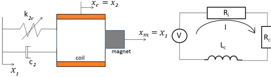
Figure 4: Coupled system: mechanical and electrical representations
