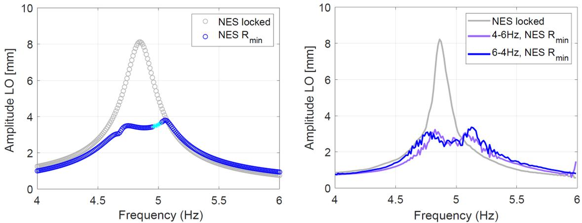
Figure 17: Evolution of the LO amplitude without and with NES +  $R_{inf}$  as a function of the frequency for  $F_e = 25$  N. The figure on the left introduces the analytical results (o blue: stable solution; + turquoise: unstable solution). The figure on the right introduces the experimental results
