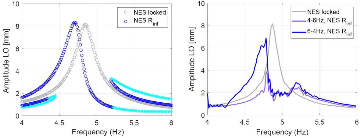
Figure 16: Evolution of the LO amplitude as a function of the frequency for  $F_e = 25$  N. The figure on the left introduces the analytical results (o blue: stable solution; + turquoise: unstable solution). The figure on the right introduces the experimental results
