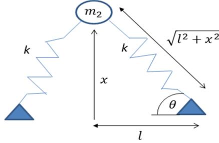
Figure 2: Springs configuration causing nonlinear stiffness
