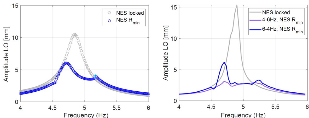
Figure 19: Evolution of the LO amplitude as a function of the frequency for  $F_e = 30$  N. The figure on the left introduces the analytical results (o blue: stable solution; + turquoise: unstable solution). The figure on the right introduces the experimental results
