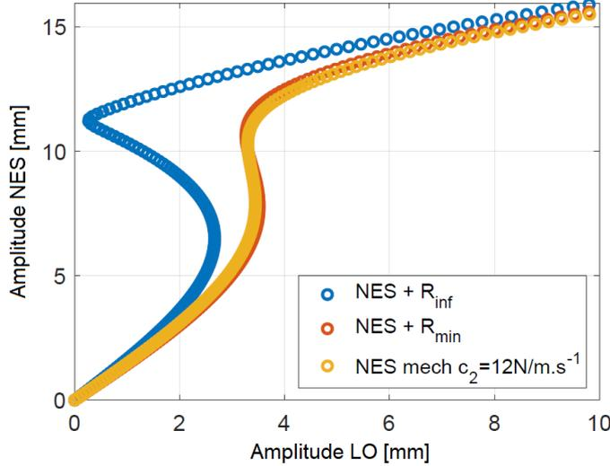
Figure 10: Slow Invariant Manifold of different NES configurations
