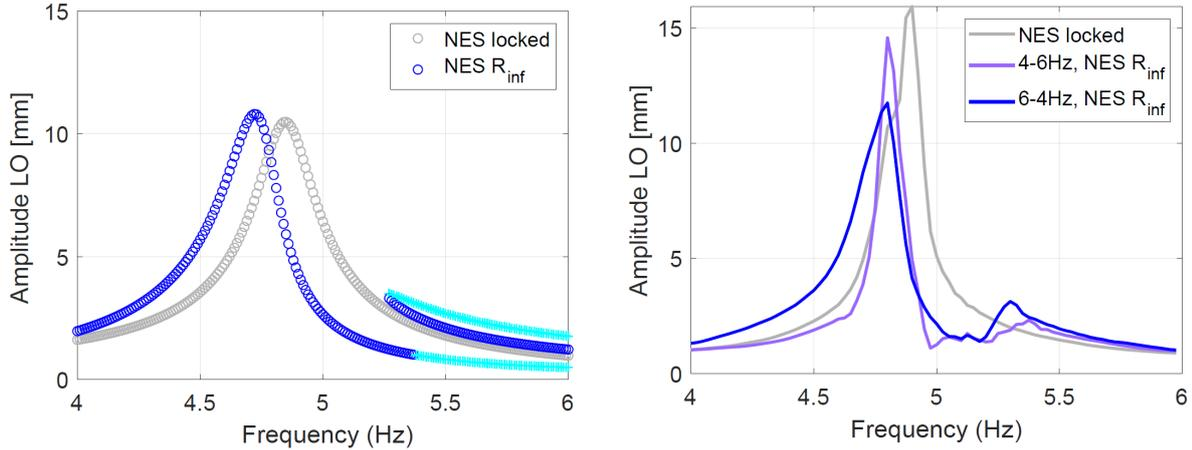
Figure 18: Evolution of the LO amplitude without and with NES +  $R_{inf}$  as a function of the frequency for  $F_e = 30$  N. The figure on the left introduces the analytical results (o blue: stable solution; + turquoise: unstable solution). The figure on the right introduces the experimental results
