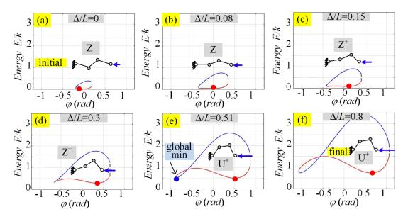
**Fig. 9** Evolution of energy- $\varphi$  curves for stable configuration for the initial "Z-configuration and changing of the manipulator shape under the loading (from Z<sup>-</sup> to U<sup>+</sup> configuration).
