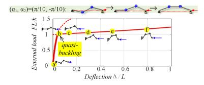
Fig. 8 Force-deflection curves for the initial "Z-configuration" and evolution of the manipulator shape under the loading.
