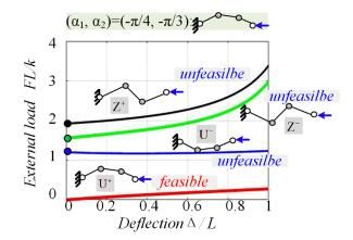
**Fig. 7** Force-deflection curves computed for different shapes and the same initial "U-configuration" corresponding to four possible equilibriums with the feasible shape  $U^+$  and unfeasible shapes  $(U^-, Z^+, Z^-)$ .
