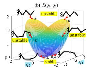
**Fig. 16** The energy function  $E(q_1, q_2)$  and static equilibriums for  $\delta x=0.5L$ ,  $\delta y=0$ .
