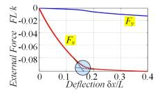
**Fig. 14** Force-deflection curves  $F_x(\delta x)$ ,  $F_y(\delta x)$  for initial Z-shape (end-effector deflection  $\delta y=0$ ; q4>0).
