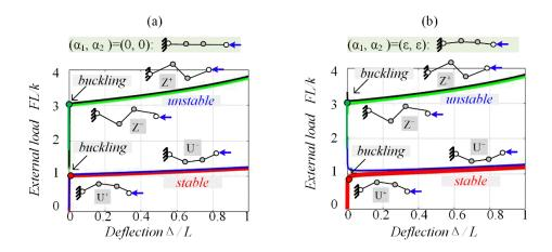
**Fig. 5** Three-link manipulator: force-deflection curves for the initial "straight" and "quasi-straight" configurations and four possible equilibriums with stable shapes  $(U^+, U^-)$  and unstable shapes  $(Z^+, Z^-)$ .
