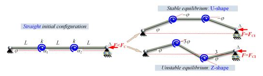
Fig. 6 Evolution of the mechanism shape after the buckling: two possible equilibriums with U-shape and Z-shape.
