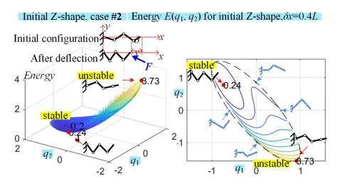
**Fig. 13** The energy function  $E(q_1, q_2)$  and manipulator equilibriums of initial Z-shape configuration (end-effector deflection  $\delta x/L=0.4$ ,  $\delta y=0$ ; q4>0).
