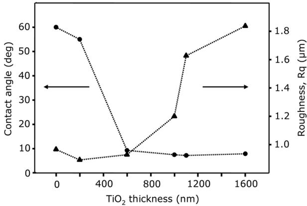
**FIGURE 2.** Variation of the water contact angle and variation of the roughness with increasing TiO<sub>2</sub> film thickness.
