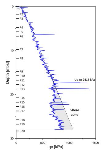
Figure 3. Sensor depths of the PZC piezometer shown together with the tip resistance (qc) obtained from site PFM12-S2 showing the presence of a well-formed shear zone (gray-shading) below 22 m below the seafloor (mbsf). Peak values of qc correspond to the presence of sandy/silty layers.
