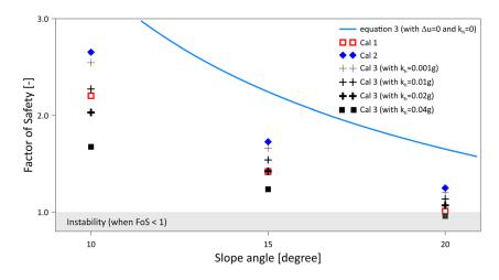
**Figure 13.** Calculated FoS at the depth level of PZC/P18 sensor (25.75 mbsf) as a function of slope angle, excess pore pressure, and horizontal acceleration. The three-case calculations (cal 1:  $\Delta u = 64$  kPa, cal 2:  $\Delta u = 40$  kPa, and cal 3:  $\Delta u = 44$  kPa) shown in Figure 12 are considered for three slope angles (10°, 15°, and 20°). For cal 3, we considered four different accelerations (0.001, 0.01, 0.02, and 0.04 g).
