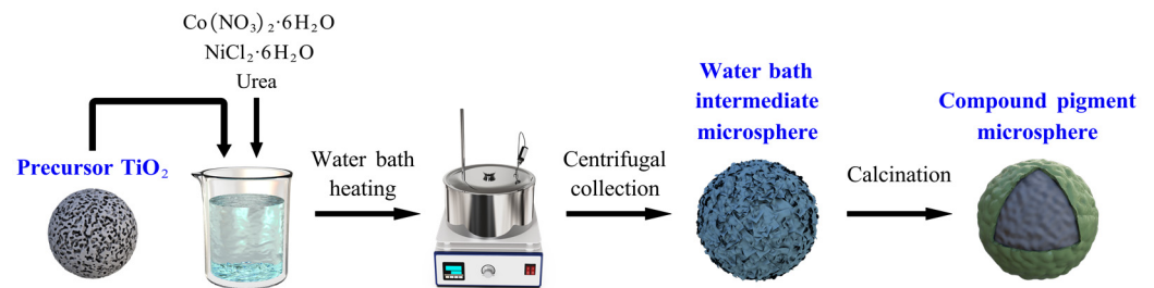
Figure 1. Process diagram for the preparation of composite pigment powders.
