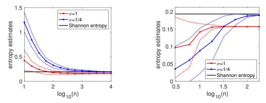
Figure 1: Negative entropy estimation from 20 replications (mean and standard deviation) for two values of the kernel bandwidth  $\sigma$ , as *n* increases. Left: from i.i.d. samples (method from Section 5.1). Right: from kernel integrals evaluated as uniform samples (method from Section 5.4). As expected we estimate the kernel entropy (limit when *n* tends to infinity) from above on the left plot, and from below on the right plot, with a faster convergence rate on the right plot.
