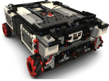
Figure 2: The EV3 Lego mindstorms robot, equipped with Mecanum-like omnidirectional wheels.
