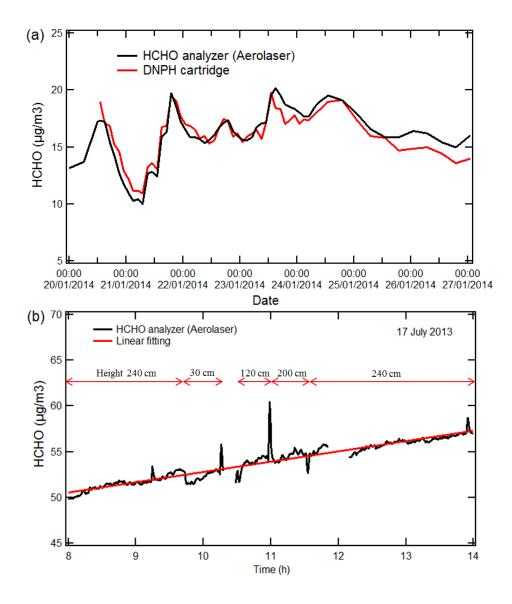
**Fig. 1.** Validation of HCHO data: (**a**) comparison of HCHO concentration measured by HCHO monitor and by DNPH-Cartridges during the period from January 20 to January 27, 2014 at Polytech University (**b**) Variation of HCHO concentration with sample height at Polytech University.
