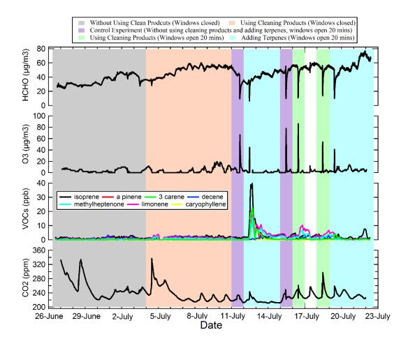
Fig. 5 Variation of indoor formaldehyde, VOCs and  $CO_2$  at the university during the period from June 26 to July 22, 2013. The part marked in white corresponds to measurements during a day without specific experiment.
