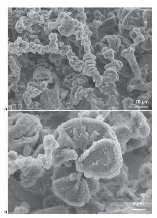
2 a Interconnected strings of graphite crystallites as observed in SEM on a deeply etched sample; b Termination of a graphite string with an incomplete graphite nodule
