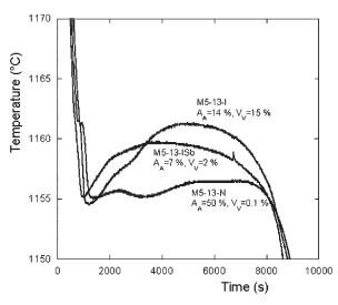
4 Comparison of the cooling curves obtained at the thermal centre of the three blocks of trial M5-13 with A<sub>A</sub> and V<sub>V</sub> values indicated
