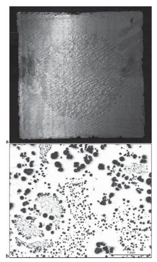
1 a Central section of a cast block with the zone affected by CHG appearing with darker contrast; b Optical micrograph of a heavy section SG cast iron part showing dendrite-like ex-austenite with large nodules embedded in, cells of CHG and areas of usual SG microstructure
