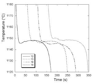
3 Cooling curves recorded on the TA cups for melts with post-inoculation
