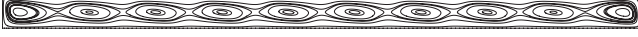
FIG. 7. A typical instantaneous streamline pattern for Le=100 , \psi=0.1 , Ra=28 during the oscillation.
