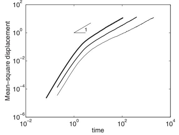
FIG. 3. Mean-square displacement  $\langle [x_2(t) - x_2(0)]^2 \rangle / (2a^2)$  vs time ( $t\gamma^{-1}$ ) in log-log scale. The lines correspond to  $\text{St}=1$  and  $\phi = 5, 15, 30\%$ , respectively, from the bottom to the upper line. The slope 1 shows the linear regime of temporal evolution.
