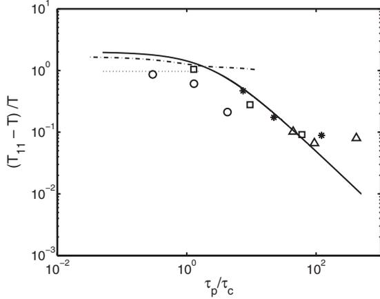
FIG. 2. Kinetic stress difference  $(T_{11}-T)/T$  vs  $\tau_p/\tau_c$ . Solid line: theoretical prediction for the ignited state. Dotted and dotted-dashed lines: quenched theory for  $St=1$  and  $St=3.5$ , respectively. Symbols: numerical results ( $\Delta$ ,  $*$ ,  $\square$ ,  $\circ$  correspond, respectively, to  $St=10, 5, 3.5$ , and  $1$ ).
