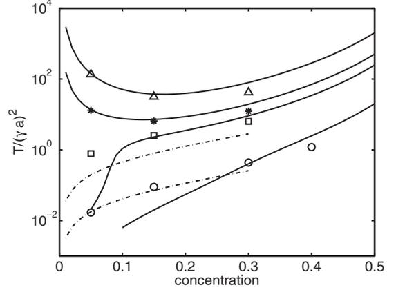
FIG. 1.  $T/(\gamma a)^2$  vs  $\phi$ . Symbols: numerical results ( $\Delta$ ,  $*$ ,  $\square$ ,  $\circ$  correspond, respectively, to  $St=10, 5, 3.5$ , and  $1$ ). Solid lines: prediction of the ignited theory (from top to bottom:  $St=10, 5, 3.5$  and  $1$ ). Dashed-dotted lines: quenched theory of [20] multiplied by  $2g_0$  (upper:  $St=3.5$ , lower:  $St=1$ ).
