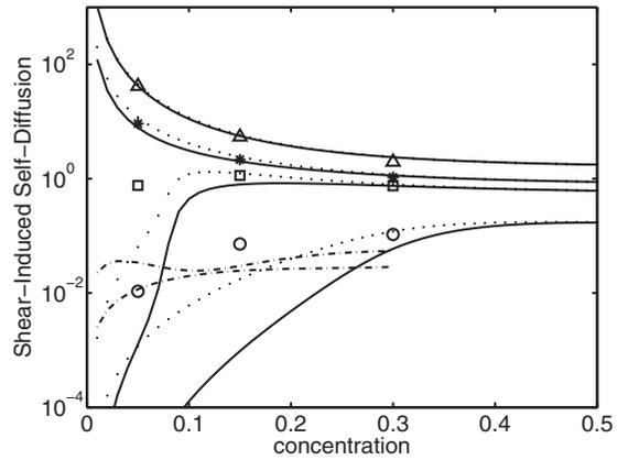
FIG. 7. Self-diffusion coefficient  $D_{22}/\gamma a^2$  vs solid volume fraction. Symbols: simulation results ( $\Delta$ ,  $*$ ,  $\square$ ,  $\circ$  correspond, respectively, to  $St=10$ ,  $5$ ,  $3.5$  and  $1$ ). Theoretical predictions [Eq. (9)] using  $T_{ij}$  from the ignited (solid lines) and quenched (dotted-dashed lines) theories, respectively, (similar to Fig. 1). Dotted lines:  $D_{iso}$  (from top to bottom:  $St=10$ ,  $5$ ,  $3.5$ , and  $1$ ).
