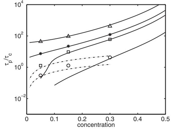
FIG. 6. Time scale ratio  $\tau_p/\tau_c$  vs solid volume fraction for different Stokes numbers. For caption see Fig. 1. The expressions used for the solid and dotted-dashed lines are, respectively,  $\tau_c = \frac{a\sqrt{\pi}}{12\phi g_0 T}$  and  $\tau_c = \frac{\pi}{16\phi\gamma}$ .
