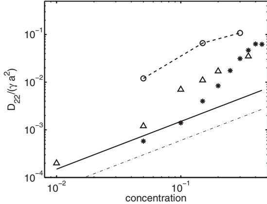
FIG. 8. Comparison of the self-diffusion coefficients  $D_{22}/\gamma a^2$  for  $St=1$  with reference results for  $St \ll 1$ .  $-\circ-$ : our numerical results for  $St=1$ . Solid line: theory of [23]. Symbols \* and  $\Delta$ : results of [21,2], respectively. Thin dotted-dashed line: prediction based on [6].
