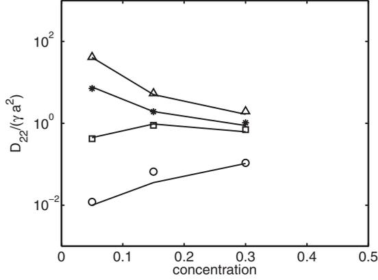
FIG. 4.  $D_{22}/\gamma a^2$  vs  $\phi$ . Symbols: numerical results (see Fig. 1). Lines: *a priori* prediction of the model [Eq. (9)] with inputs ( $T_{ij}$  and  $\tau_c$ ) from the numerical simulations.
