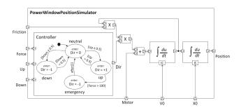
**Fig. 16** Partial model of a power window in a car. The first CBD Block continuously computes in which direction the Window (motor) moves, transmitting the information to the second Block, which effectively realises the movement
