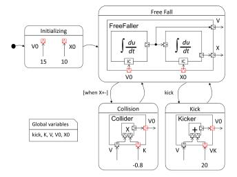
**Fig. 15** Model of the Kickable Bouncing Ball: after Initialising the necessary state variables, the ball is in FreeFall, following Netwton's Free Fall Law, then Colliding, thus bouncing. Sometimes, the ball gets Kicked, allowing it to momentarily gain upward speed. The Global Variables are shared by the CBD inside the States
