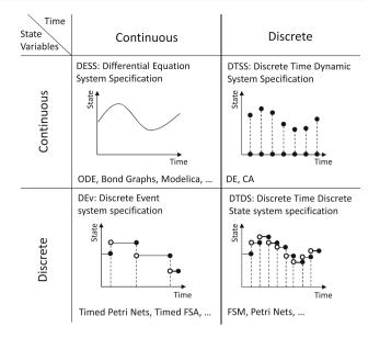
Fig. 5 Classification of modelling abstractions for dynamic systems according to the nature of the *time* and *state* variables [72,79]
