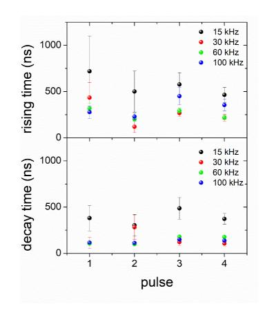
Fig. 3: Time constants for a) the increasing and b) the decreasing strain response of the PLZT12 thin film during the application of PUND pulse sequences with frequencies ranging from 15 to 100 kHz.
