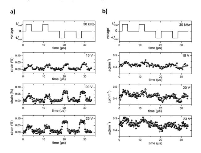
Fig. 1: a) Strain transient and b) transient of the peak width  $\Delta q$  of the PLZT 110 Bragg reflection for a PUND pulse sequence with a frequency of 30 kHz and peak voltages of 15, 20, and 23 V. Additional frequencies of 15, 60, and 100 kHz for the three different voltages of 15, 20, and 23 V are shown in Fig. S9 of the supplementary material.
