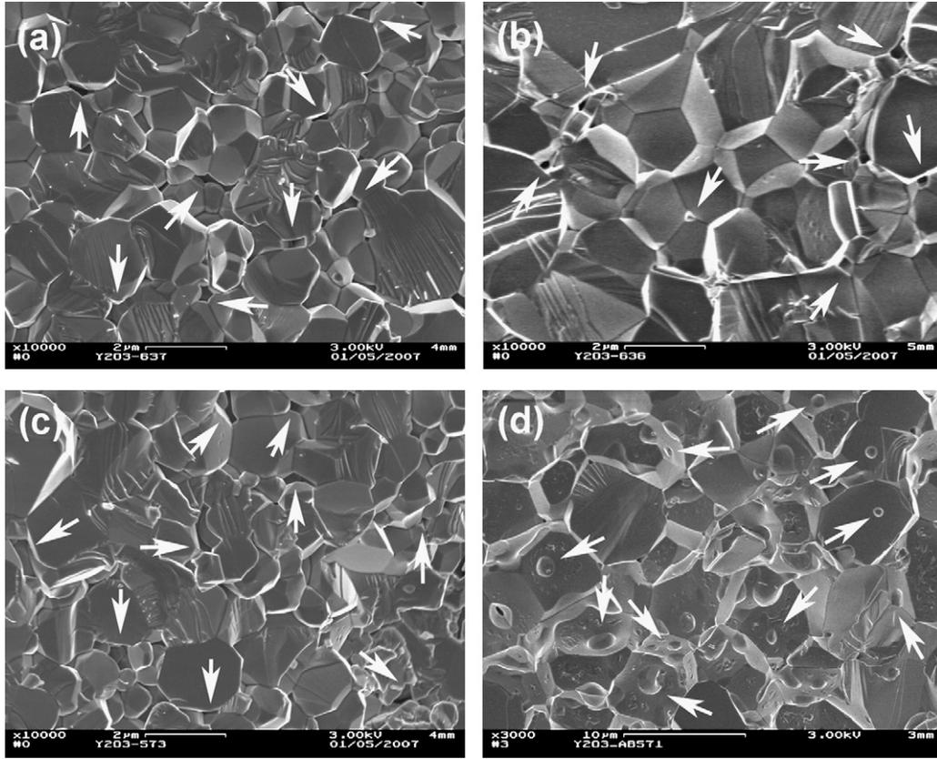
Fig. 6. SEM images from the fracture surfaces of  $Y_2O_3$  specimens after SPS at (a) 1100 °C, (b) 1200 °C, (c) 1300 °C, (d) 1400 °C. The pores at the grain junctions in (a) to (c) and on grain boundaries in (d) were arrowed.
