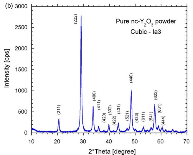
Fig. 1. (a) Bright-field TEM image showing the  $\text{Y}_2\text{O}_3$  nanocrystallites agglomerated as sub-micrometer powder particles. (b) X-ray diffraction spectrum showing the  $\text{Y}_2\text{O}_3$  cubic symmetry.
