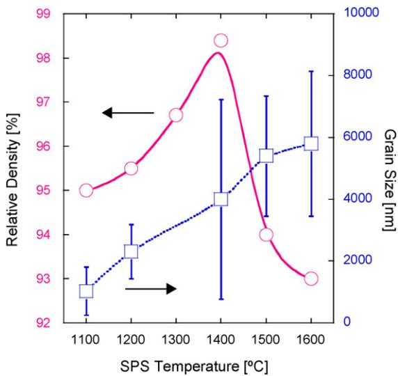
Fig. 4. Relative density and average grain size versus the SPS temperature for 5 min and 100 MPa, using the heating rate 180°C min<sup>-1</sup>.
