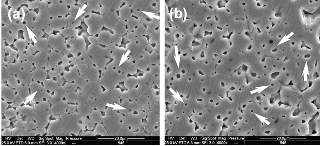
Fig. 7. SEM images from the polished and chemically etched  $Y_2O_3$  specimens after SPS at (a) 1500 °C, and (b) 1600 °C. The residual pores located at the grain boundaries and within the grains, the latter were arrowed.
