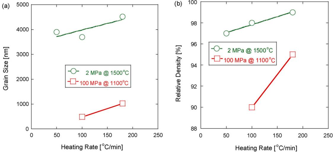
Fig. 3. Effect of heating rate at different SPS pressures and temperatures on the (a) grain size and (b) relative density of nc-Y<sub>2</sub>O<sub>3</sub>.
