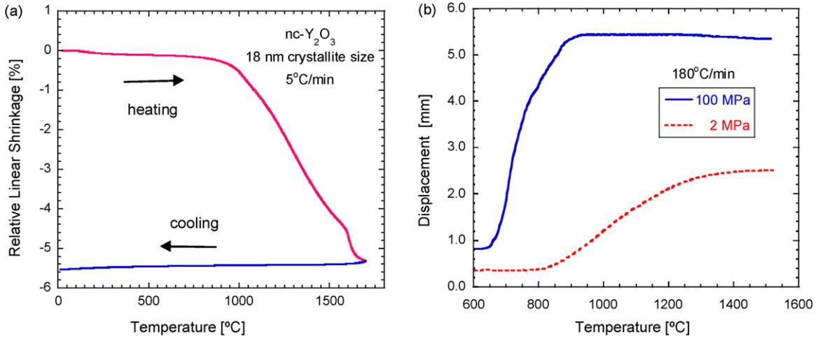
Fig. 2. Linear shrinkage of nc-Y<sub>2</sub>O<sub>3</sub> powder compact in (a) dilatometer at 5°C min<sup>-1</sup> heating rate. (b) SPS under 2 and 100 MPa load and high heating rate of 180°C min<sup>-1</sup>.
