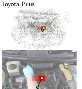
Object: negative battery cable Query: the negative battery terminal is usually black and may have a minus sign near it
