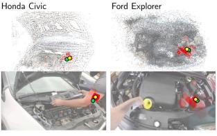
Object: positive battery cable Query: disconnect the positive cable next and secure it with a cable tie
