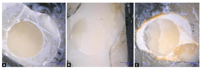
Figs 1A to C: Representative photos of numeric optical microscope of: (A) Adhesive failure (×50 magnification); (B) Mixed interfacial failure (×50 magnification); (C) Cohesive failure in composite layers (×50 magnification)
