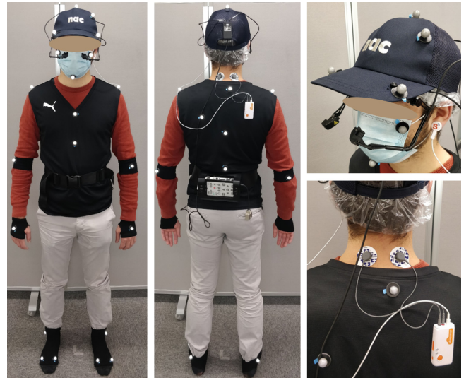
Fig. 3: Sensors setup: 27 motion capture markers, EMR eye-tracker with cap and battery bag, Shimmer3 GSR+ sensor with earlobe for PPG measurement and single-use gel-type electrodes for GSR measurements.
