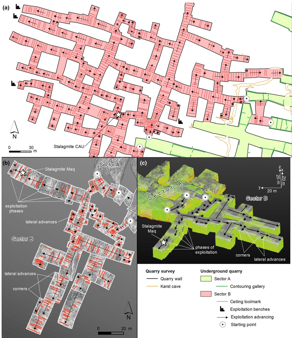
FIGURE 3 (a) West part of the quarry map showing ceiling toolmarks, excavation progress and examples of exploitation phases and corners. (b) Ceiling toolmarks shown by the high-resolution 3D model, indicating the direction of the exploitation in Les Maquisards part. (c) 3D geometry of the galleries. The starting points of sector B are indicated (white dots) in the three sections, the positions of which are shown in Figure 2A
