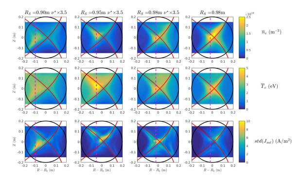
Figure 9: First row: plasma density in three GBS simulations with particle source at  $R_S = [0.90; 0.95; 0.98]$  m and increased collisionality. The center of the source is identified by a vertical dashed line. The fourth column shows the reference GBS simulation with collisionality set to the Braginskii value. Second row: the same for electron temperature. Third row: standard deviation of the ion saturation current.
