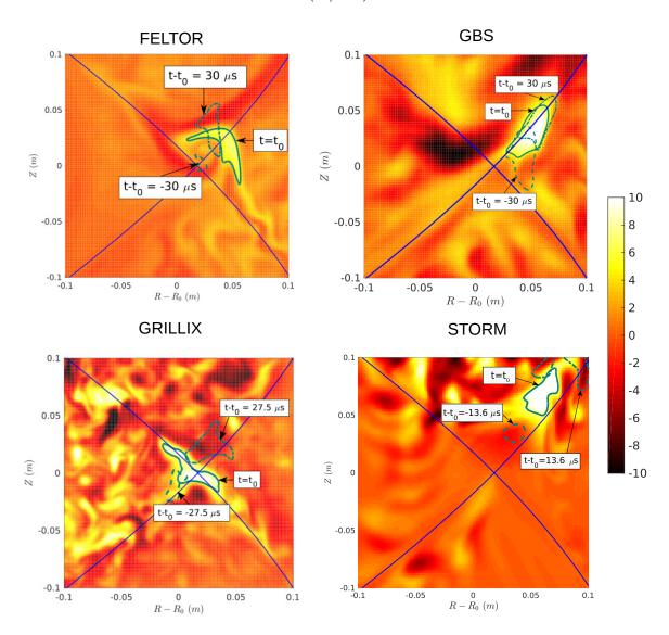
Figure 7: Snapshot of the ion saturation current density fluctuation  $\delta J_{sat} = J_{sat} - \overline{J}_{sat}$  (A/m<sup>2</sup>) at a chosen time  $t_0$ , different for each of the codes (zoom around the X-point region). Dashed, solid and dashed-dotted green lines indicate the blob contour at three different time frames, indicated on the figures. The separatrix is represented in blue.
