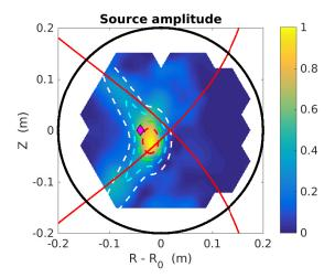
Figure 4: Measured particle source, normalized to its maximum. White, cyan, green and red dashed lines represent the contours of the fitting function  $f_S = 0.2$ , 0.4, 0.6 and 0.8, respectively. The magenta diamond indicates the position at which simulations are meant to match electron density and temperature.
