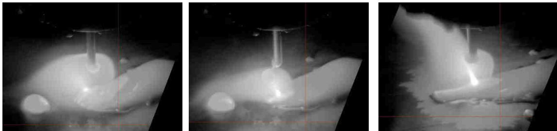
Figure 4 – Behavior of the liquid deposit in the presence of projection (1007 synergic line / WFS = 4 \text{ m.min}^{-1} / TS = 0.36 \text{ m.min}^{-1} )
