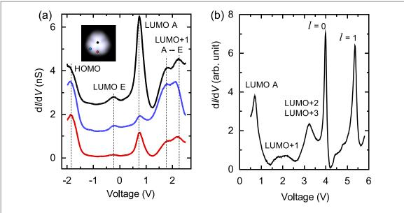
**Figure 2.** (a) Constant-height dI/dV spectra acquired for tip positions marked by the dots in the STM image in inset  $(2.3 \times 2.3 \text{ nm}^2, V = 2.2 \text{ V})$ . (b) Constant-current dI/dV spectrum for the tip positioned above the center of  $C_{60}$  (I = 1 nA).
