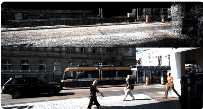
Fig. 13. Synthetic image generation of station sequence: top image is the rendered static scene imaginary by using the reconstructed static map. By comparing to the bottom real camera captured image, we notice that large moving objects (such as the moving car and train) are correctly detected and removed.
