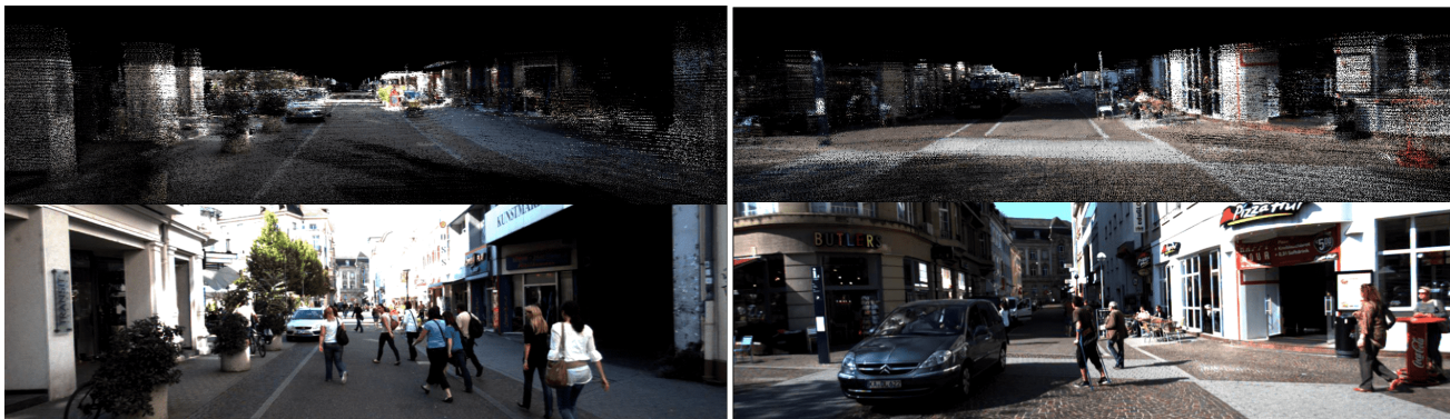
Fig. 12. Synthetic image generation of market sequence by using the reconstructed static map. Top images illustrate the static scene imaginary of the market area, while the bottom images are "contaminated" by the moving car and the numerous walking pedestrians.
