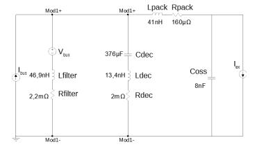
Fig. 10. Complete model circuit of power converter ONIX 671 for Cdec =  $8 \times 47 \mu F$ . The operating point is  $V_{bus} = 800 V$ ,  $I_{ex}$  is a square waveform with 0.5 duty cycle swinging from 0 to 1000A, and  $I_{bus} = 500 A$  to provide the average value of  $I_{ex}$ .
