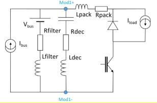
Fig. 8. Simplified equivalent electrical circuit of Fig. 7 (coupling not displayed), used in a chopper cell to focus on switching events.  $I_{bus}$  represents the current delivered by the power source, and Cfilter has been replaced by a DC voltage source  $V_{bus}$ . The load is modeled by a simple DC current source  $I_{load}$ .
