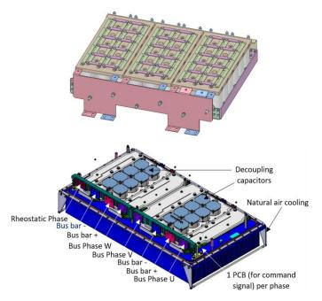
Fig. 3. Alstom converter ONIX 671. Top: 3x18 Electrolytic capacitor association (filter capacitor). Bottom: 4 power bus bars (2 used for 2 legs), 8 decoupling capacitors and 12 IGBT dual power modules 1.7kV / 1200A (3 per phase).
