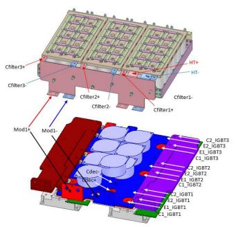
Fig. 6. Identification of the common points Mod1 + and Mod1- on the bus bars that connect the filter capacitors (top) and the bus bars that connect the decoupling capacitors and the semiconductors (bottom).
