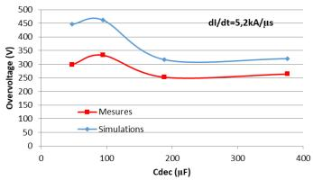
Fig. 14. Simulation results of the model in Simplorer simulation (♦) and test bench measurements (■) for two switching speeds.
