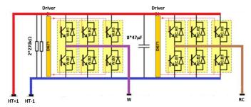
Fig. 4. Electrical schematics of phase W and rheostatic leg of power converter ONIX 671 from Alstom.
