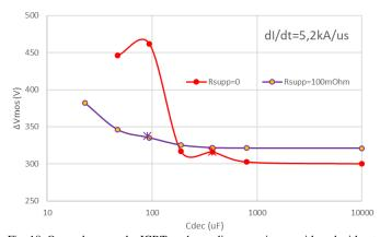
Fig. 18. Overvoltage on the IGBT vs decoupling capacitance with and without a  $100~\text{m}\Omega$  series resistance Rsupp (Simplorer simulations).
