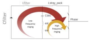
Fig. 1. Simplified switching cell and resonant circuits.
