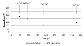
Fig. 13. IGBT overvoltage from Alstom test bench, in function of the decoupling capacitor value for two switching speeds (4.4kA/µs and 2.5kA/µs).
