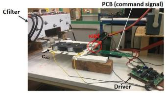
Fig. 11. Experimental bench using ONIX 671 power converter.
