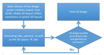
Fig. 19.Illustration of the proposed optimal sizing method inside a full 3D layout design process.
