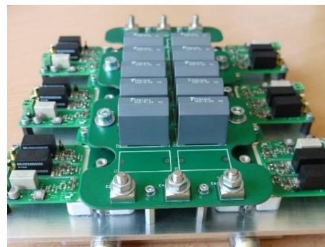
Fig. 19. 3-Phase 10 kVA inverter developed
