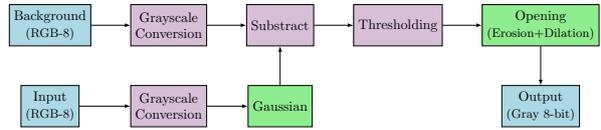
Figure 16: Pipeline for foreground extraction using **algorithms** and **views**.
