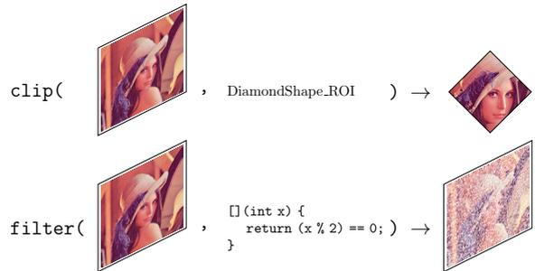
Figure 9: Clip and filter image adaptors that restrict the image domain by a non-regular ROI and by a predicate that selects only even pixels.
