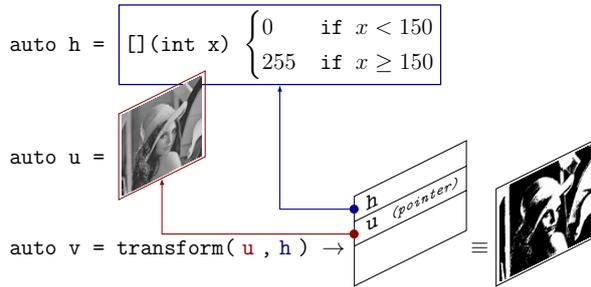
Figure 8: An image view performing a thresholding.
