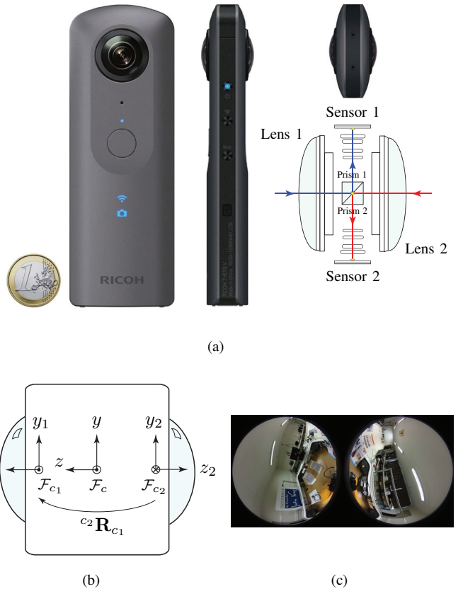
Fig. 1. (a) Front, side and top view of a twin-fisheye camera, the Ricoh Theta V (image courtesy of Ricoh), and schematic of the optical system with the two fisheye lenses, prisms and CMOS sensors; (b) \mathcal{F}_c is the camera frame, and \mathcal{F}_{c_1}, \mathcal{F}_{c_2} , the reference frames associated to the two fisheye lenses (top view); (c) Example of dual-fisheye image taken by the Ricoh Theta V: the left and right sub-images correspond to the two fisheye lenses.
